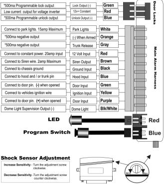
\*500ma outputs are low current and are designed to activate relays
